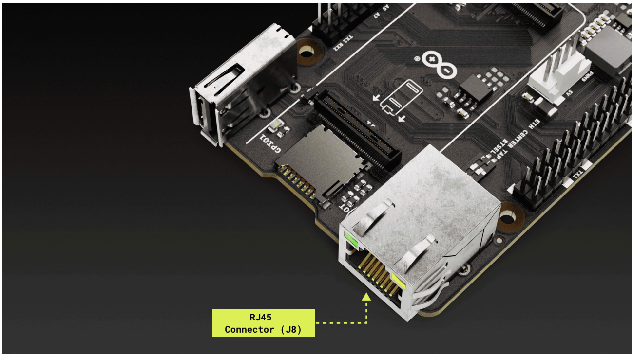
Figure 11. RJ45 connector of the Portenta Hat Carrier
